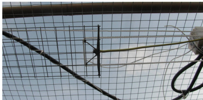
Figure 5: Radiator with feed line.
