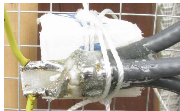
Figure 4: Balun implementation, mesh size = 12.7 mm.
